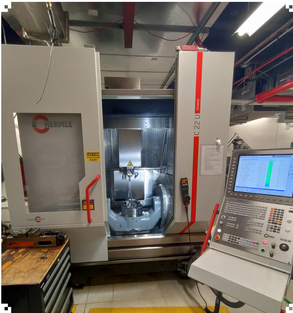
The PIT's Hermle C22U 5-Axis milling machine allows the PIT engineering staff to create parts that would otherwise be impossible or prohibitively expensive to make elsewhere.
