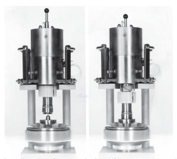
Centrifuge rotor designed by Henri Beaufay, constructed at the Rockefeller University instrument shop by Nils Jernberg for Christian de Duve, circa 1965. Rotor shown in open (left) and closed positions (right). From the Rockefeller University Merrill Chase historic scientific instrument collection, accession number 232.
